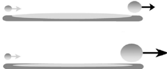
Figure 3. Comparison of the performance of two pavements with different subgrade soils
