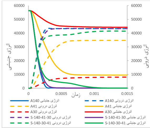
Figure 8 - Internal energy and kinetic energy diagram at a speed of 540 m/s
